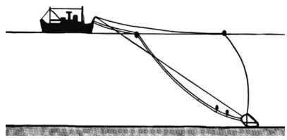
**Figure 1.** Deployment of the towed photographic sledge. From: Holme & Barrett (1977).
